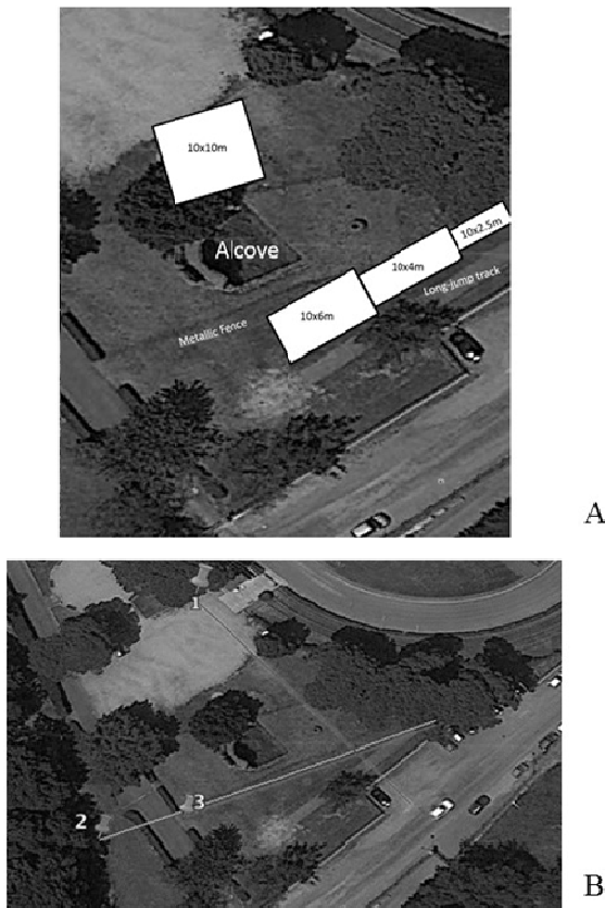
Figure 2. In this figure, the locations of the 4 GPR grids (a) and the three ERT profiles (b) are visible. Note that tomographic profiles 1 and 2 are 64-m long, whereas tomographic profile 3 is 48-m long.
